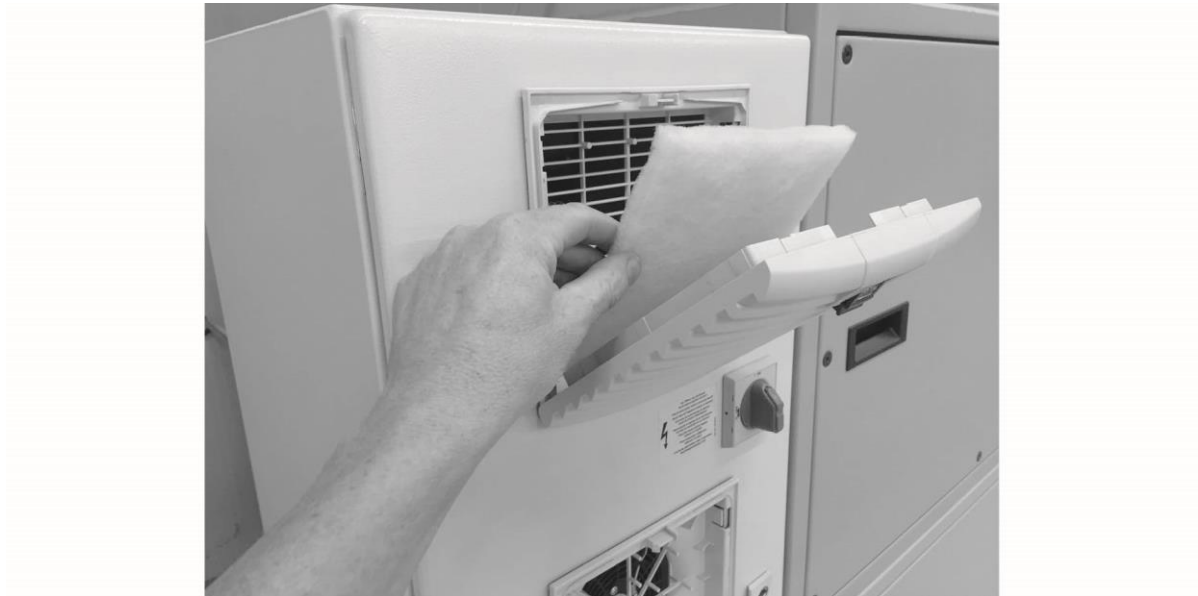
Fig. 39: Filter replacement in control cabinet
