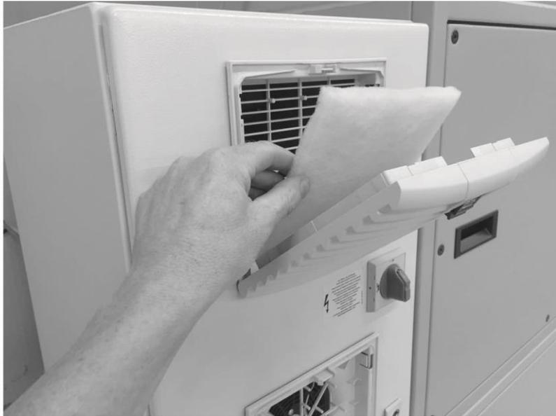
*Fig. 96: Filter replacement in control cabinet*
