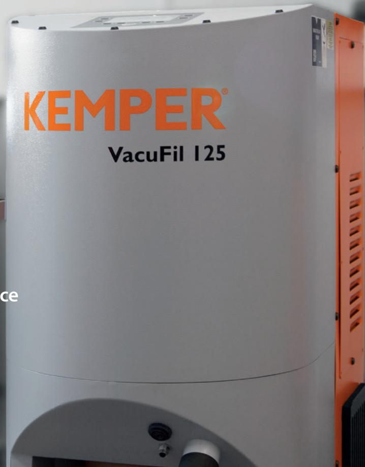
The **VacuFil 125** single-place high vacuum extraction unit for large quantities of welding fumes and dust is ideally suited for permanent use for torch-integrated extraction during welding due to its automatic filter cleaning. A side channel blower for vacuum generation ensures robust performance for industrial users. The automatic extraction capacity regulation ensures the optimum operating point for a wide variety of flue gas extraction torches.
