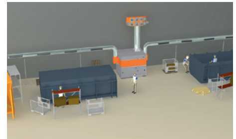
Extraction capacity: 13,000 m 3 /h
